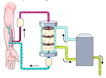
The blood flows into the dialyzer, is cleaned, and is then returned to your body. The dialyzer has a space for blood and a space for dialysis fluid.
