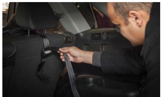
Always attach the top tether to the anchor point for that seat.
