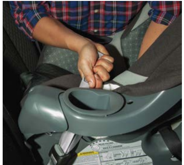
Lift the cover to get easier access to pull the strap tight.
